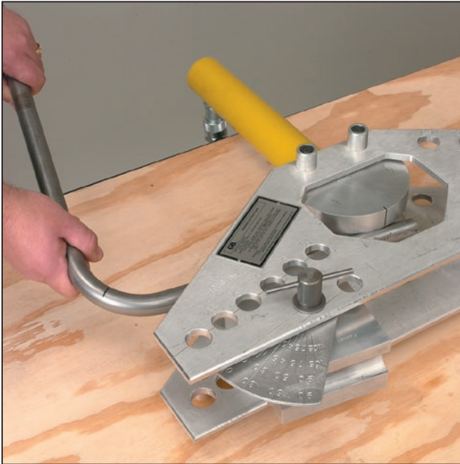
Step 9 Remove the tube. Re-orienting the slide blocks may be necessary for tube removal.
