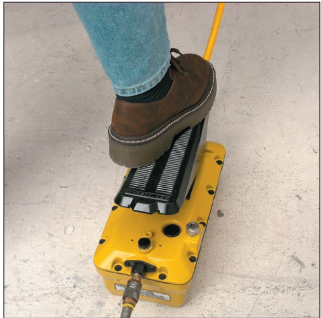
Step 8 Depress the upper portion of the foot pedal to retract the radius block.
