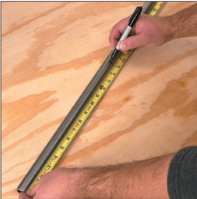
Step 3 Mark the tube to be bent with the measured distance.
