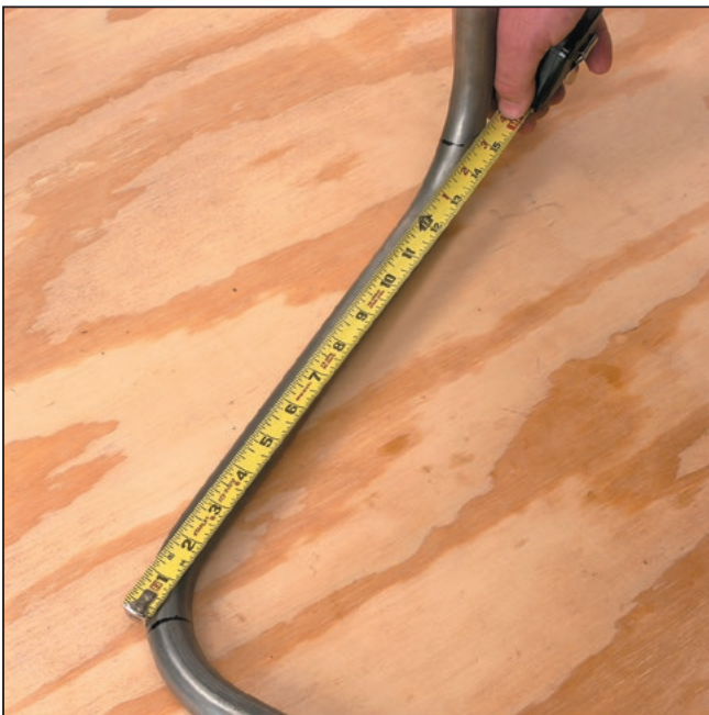
Step 11 Measure the distance from the center mark on the first bend to the center of the second bend on the original tube.
