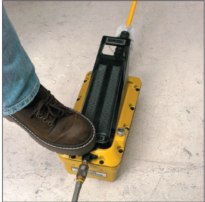
Step 6 Keeping all hands free from the moving parts of the bender, depress the foot pedal on the air/hydraulic pump to begin bending.
