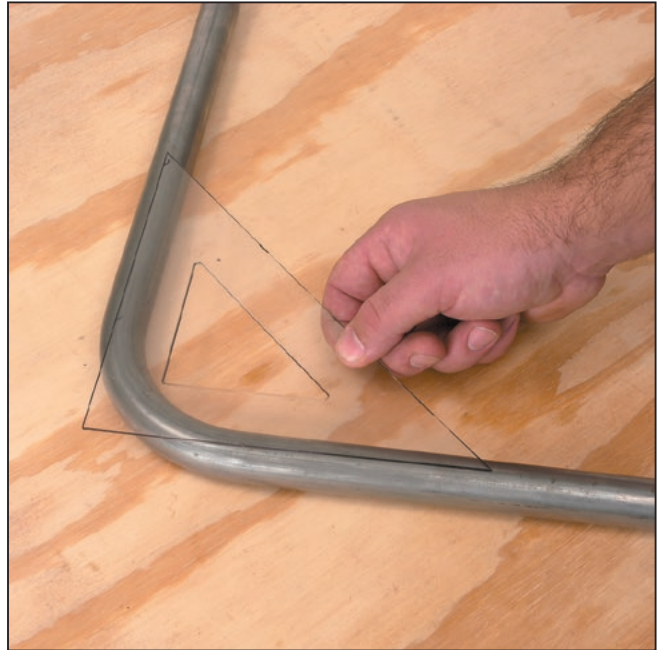
Step 10 Check the bend angle. In some cases it is necessary to overbend a few degrees to compensate for springback in the tube. If necessary, place the tube in the bender and repeat steps 4 through 9.
