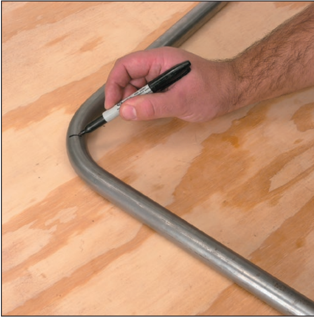
Step 1 Mark the center of all bends on the tube assembly to be duplicated.
