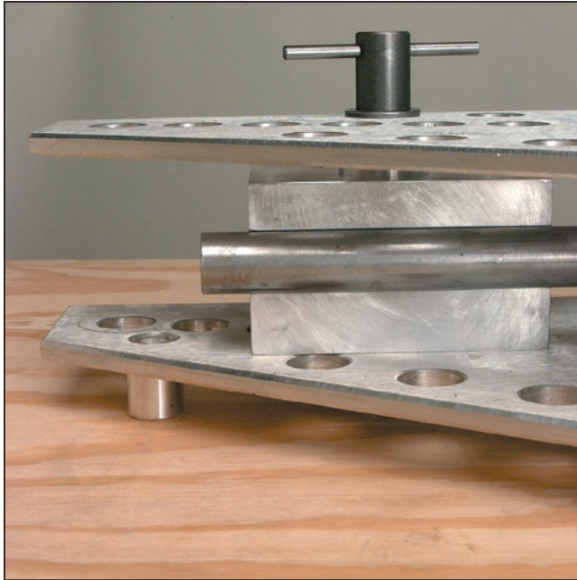
Step 5 Prior to bending, assure that there is adequate tube length to contact the slide blocks on either side.
