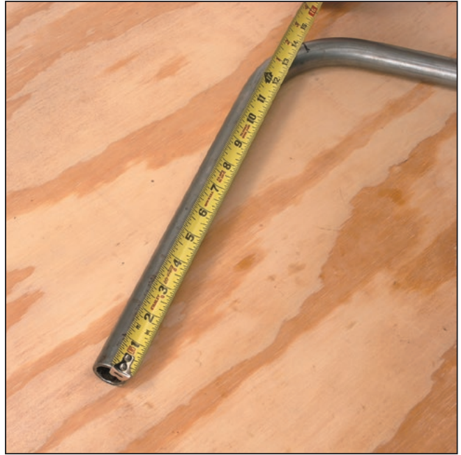
Step 2 Measure from one end of the tube to the center of the first bend. It is necessary to measure along the centerline of the tube as close as possible to achieve the correct distance.
