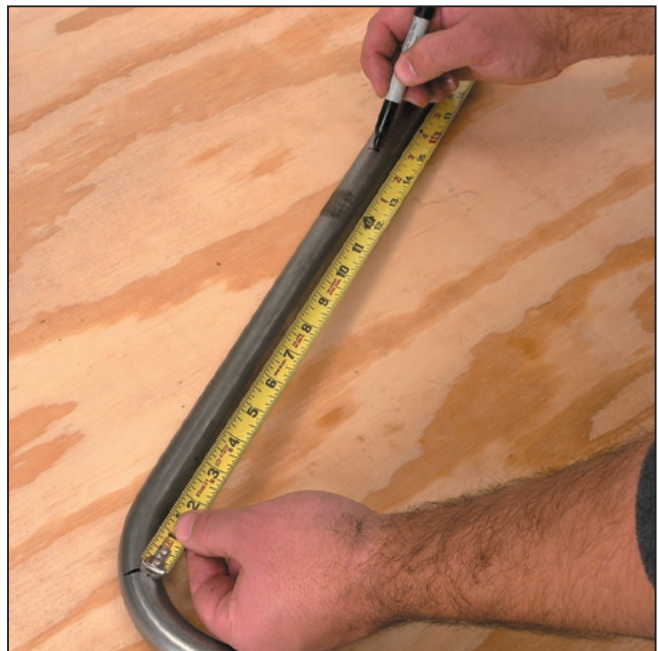
Step 12 Measure the tube to be bent from the center mark on the first bend to the distance measured on the original tube. Mark the tube.
